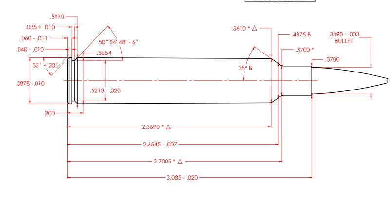
B = BASIC  $\triangle$  = REFERENCE DIMENSION  $\otimes$  = HEADSPACE DIMENSION \* DIMENSIONS ARE TO INTERSECTIONS OF LINES ALL CALCULAITONS APPLY AT MAXIMUM MATERIAL CONDITION (MMC)
