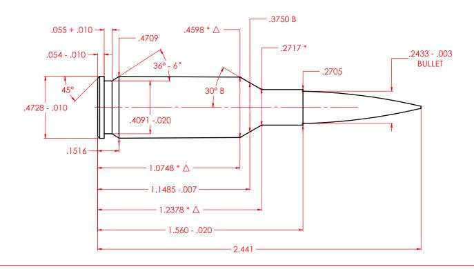
B = BASIC  $\triangle$  = REFERENCE DIMENSION  $\otimes$  = \* DIMENSIONS ARE TO INTERSECTIONS OF LINES
