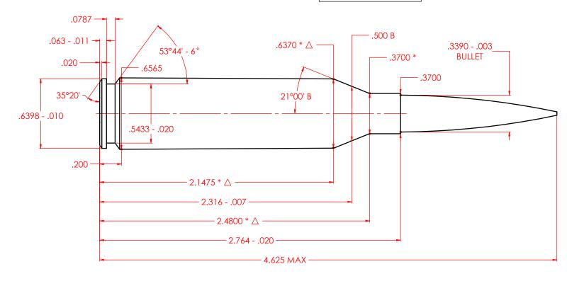
B = BASIC  $\triangle$  = REFERENCE DIMENSION \* DIMENSIONS ARE TO INTERSECTIONS OF LINES  $\otimes$  = HEADSPACE DIMENSION
